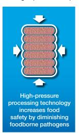
chamber and water is added before the chamber is sealed. The chamber is programmed to increase the pressure to maximum desirable level and sustain it for a set period of time. Next, the chamber is decompressed and drained, and the products are removed.
