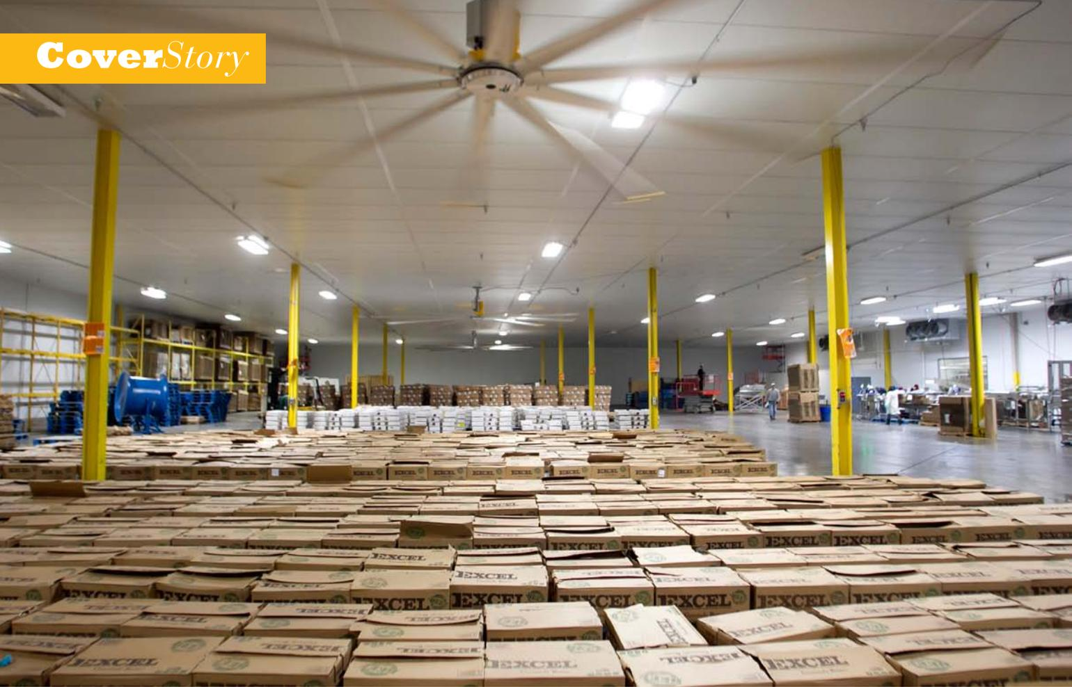
**ABOVE:** Universal Cold Storage uses a large open area in its cold-processing room to air-temper product across a single layer on the floor, moving air around the product with enormous ceiling fans and several floor fans. UCS has tempering rooms in the facility as well, but some customers request this method of tempering.
