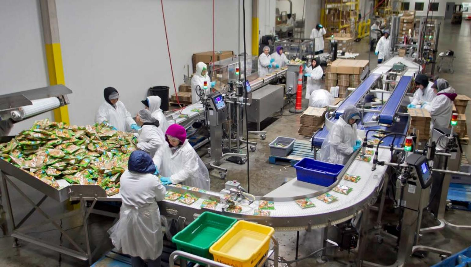
Products pour out of the HPP room at UPC's Lincoln facility, onto a conveyor in the cold-processing room, where they are inspected, labeled, boxed and palletized to be shipped out to a customer or a retail distribution center.
